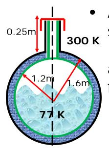
A spherical LN2 vessel (e=0.8) is as shown. The inner and outer radii are 1.2m and 1.6m respectively. Compare and comment on the heat in leak for the following cases.
