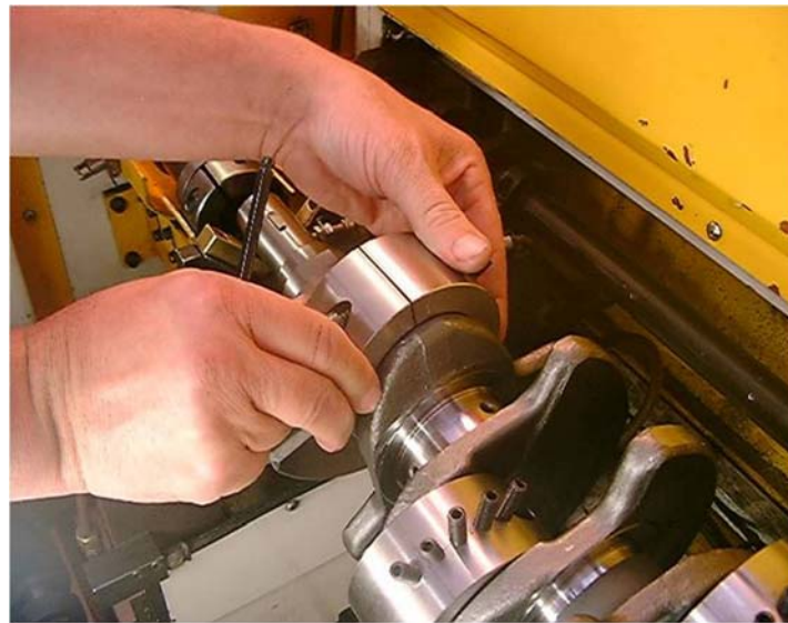
Figure 16 Ring weight installation on crankshaft – Step 2 (see online version for colours)
